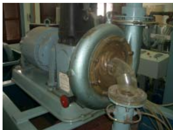
Francis (H) Turbine Model Test at EDL Training Center in Laos
