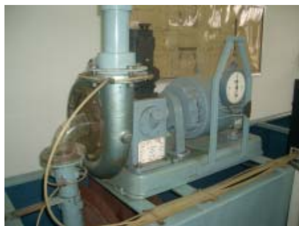
Francis (H) Turbine Model Test at EDL Training Center in Laos
