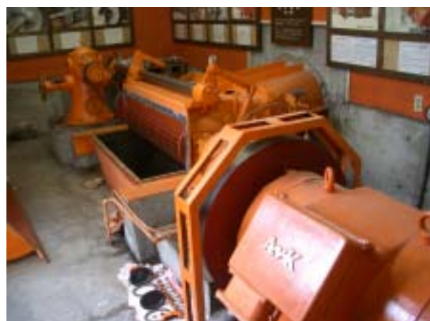
Cross Flow Turbine at Hoshino-Onsen SHP (left: No.1, 50 kW / right: No.3, 50 kW)
