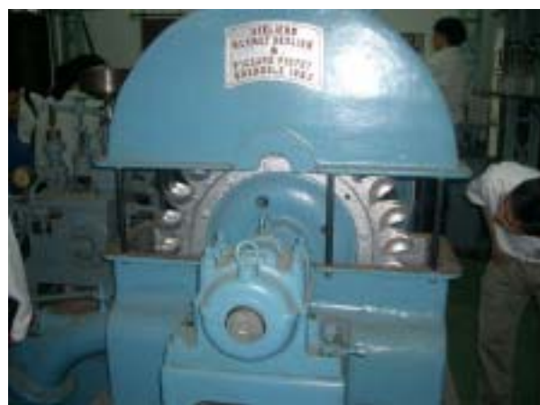
Pelton (H) Turbine at EDL Training Centre in Laos
