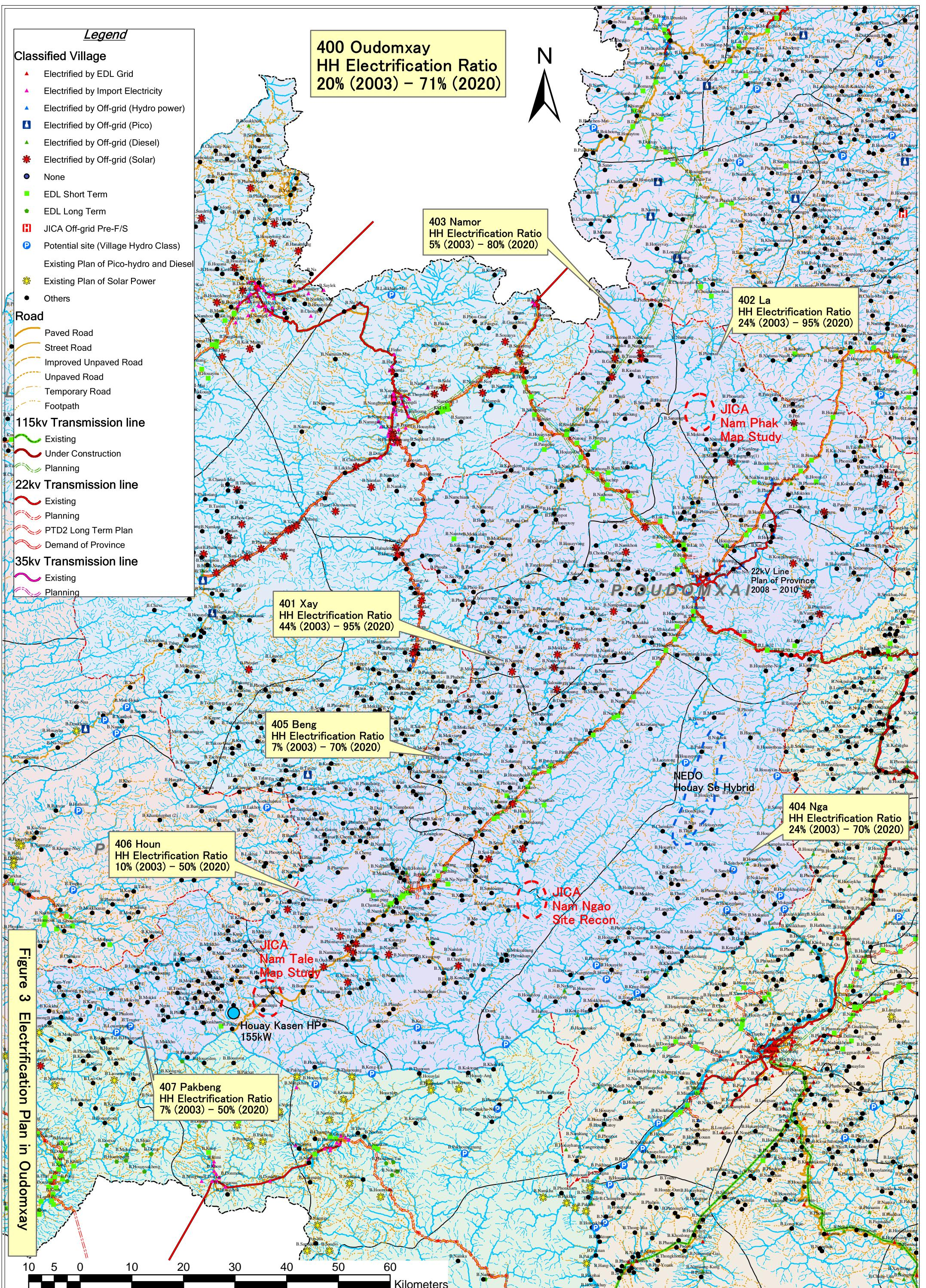
Figure 3 Electrification Plan in Oudomxay
