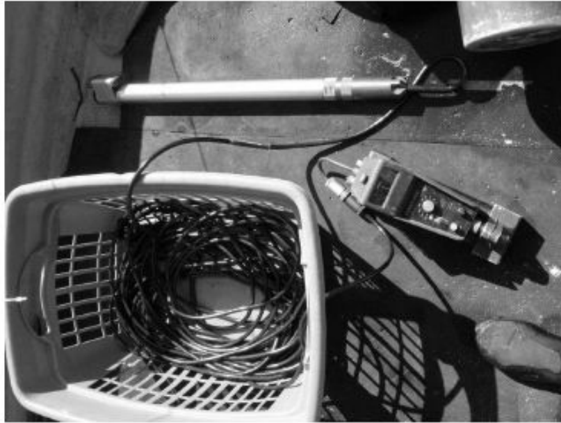
Underwater Magnetometer with 30 metres cable
