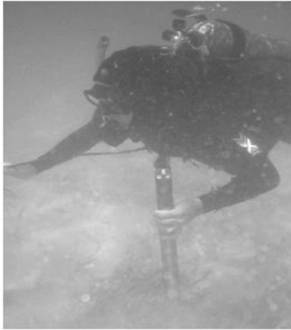
Diver using Underwater Magnetometer
