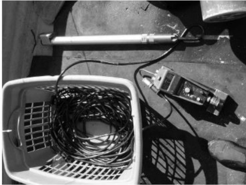
Underwater Magnetometer with 30 metres cable
