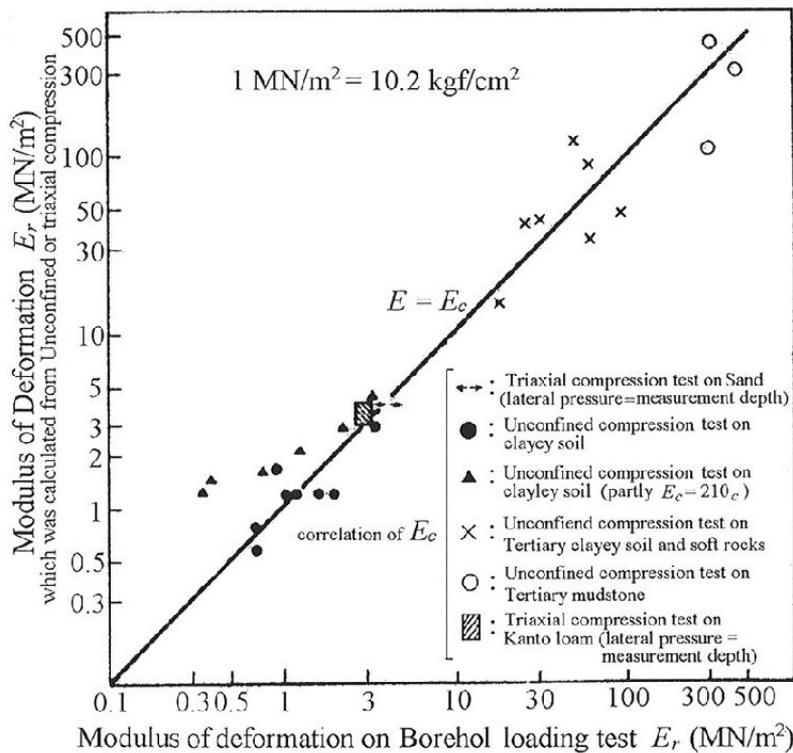
Figure 5.3.2 Relativity of modulus of deformation, obtained from Lateral loading test in borehole and Laboratory soil test
