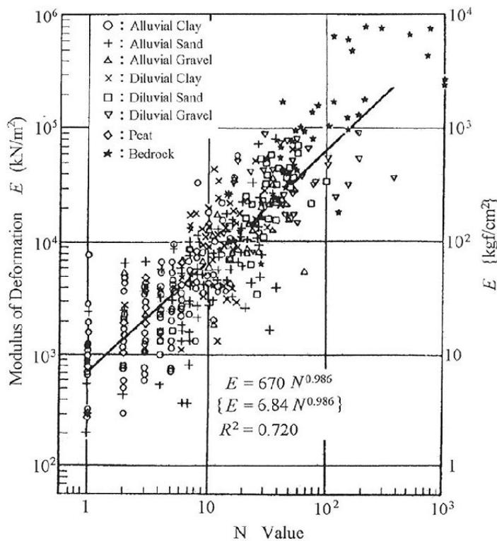
Figure 5.3.1 Relativity of N-Value and Value of modulus of deformation
