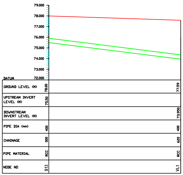
L_SECTION FOR SEWER FROM S13 TO VL1
