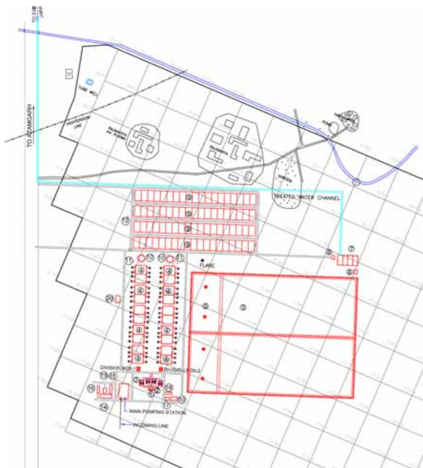
Figure 3.8 Recommended Layout of Sathwa Sewage Treatment Plant
