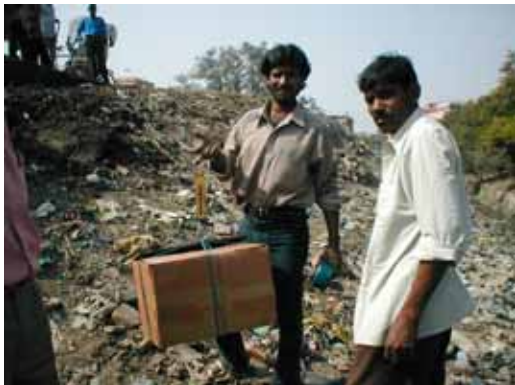
Photo 6.4 Measurement of Weight of the Solid Waste (3); measuring the weight by a spring (Assi Nala, Varanasi)
