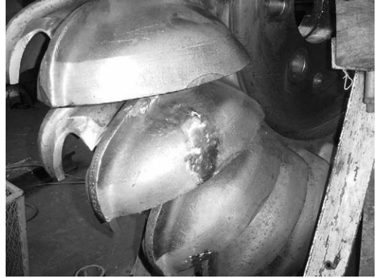
Picture 7.5 Repaired Runner Bucket of Old Laxapana Stage I
