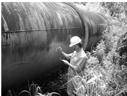
Picture 6.10 Measuring for plate thickness
