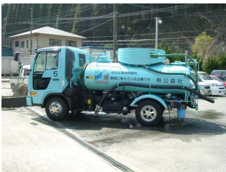
Figure M.4.5 Cleaning and Desilting Methods by Vacuum Car and Water Jetting
