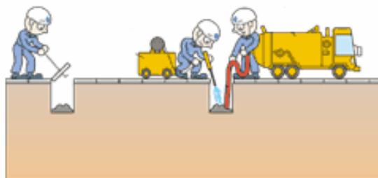
Figure M.4.5 Cleaning and Desilting Methods by Vacuum Car and Water Jetting
