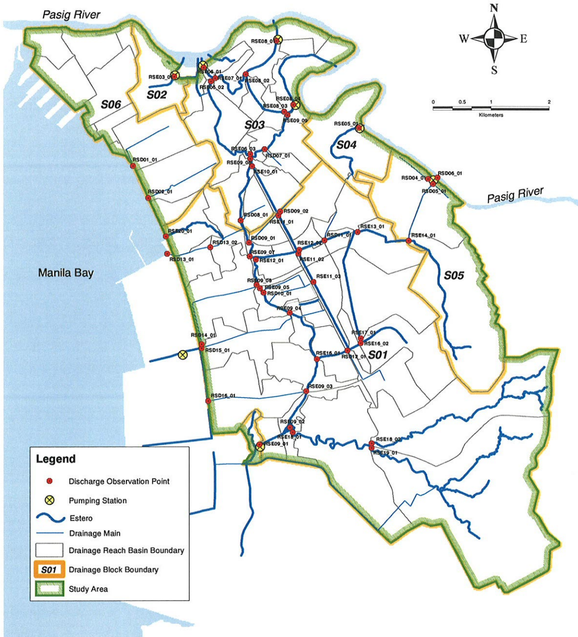
Figure E.5.7 Location of Discharge Observation Points in the Proposed Drainage Scheme (2/2)
