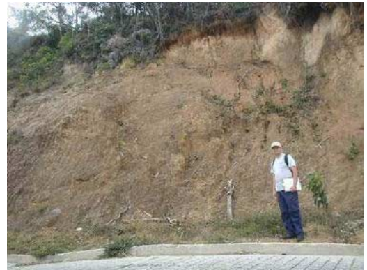
Weathering Grade V This slope consists of only Grade V
