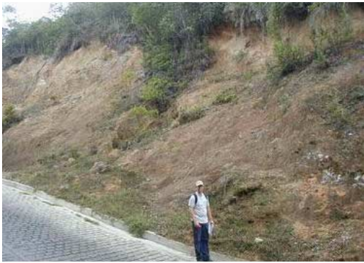
Weathering Grade VI – V Upper part of slope (whitish color) is Grade VI
