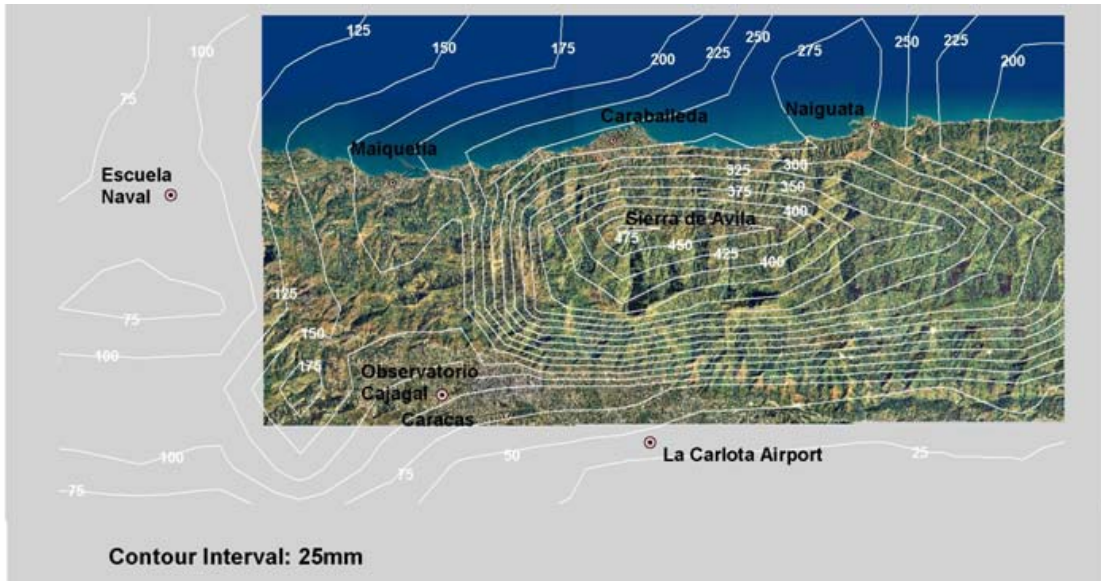
Figure 4.1.1.13(2/2) Rainfall during the Event of December 1999 in and around Caracas Valley (source: USGS)
