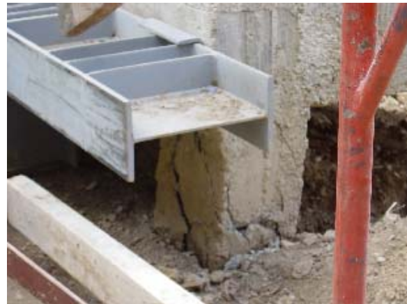
Photo 3.5.60 Model 2 Photo 3.5.61 Model 2-Shear Failure of Short Column (1)
