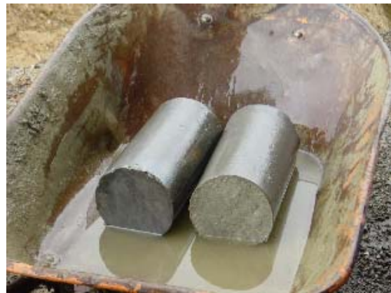
Photo 3.5.17 Concrete Test Cylinder
