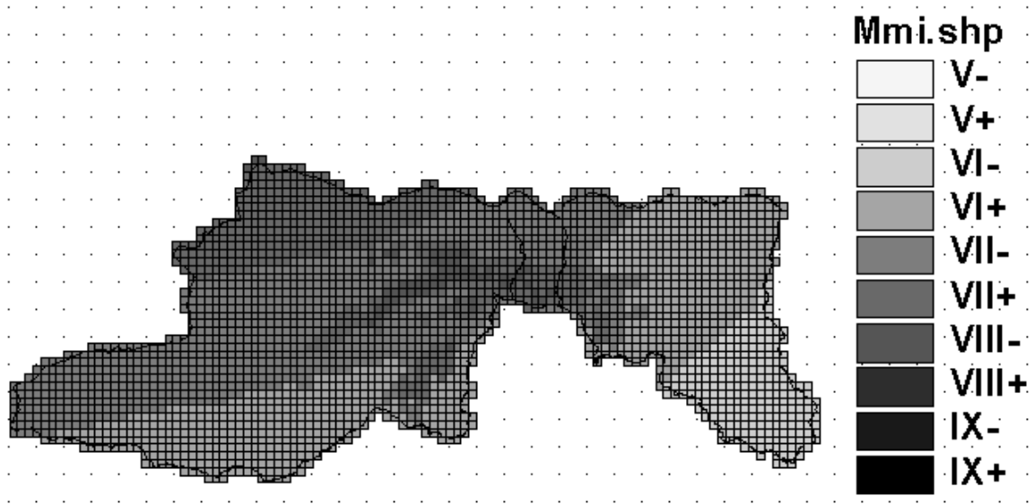
Figure 3.1.3 Estimated Seismic Intensity for the 1967 Earthquake
