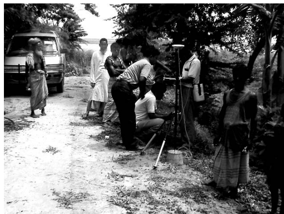
2. Check Survey of Installed Control Point by GPS
