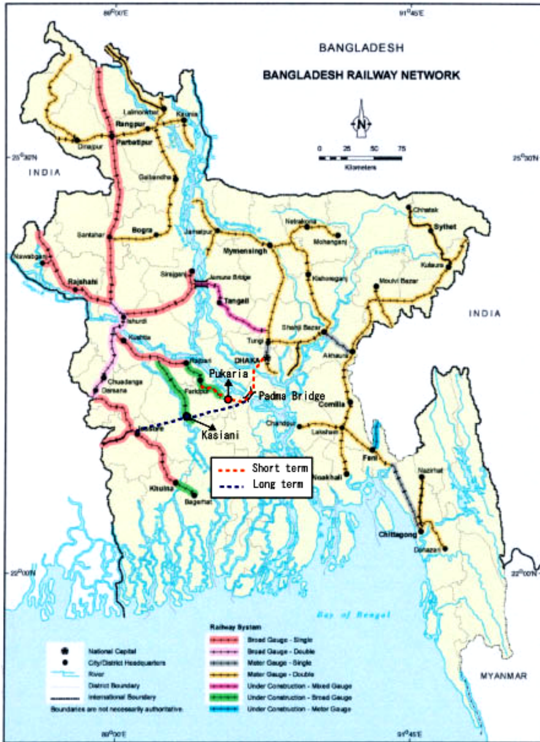
Figure 11.4.5 Conceptual Plan of Railway Trans-Padma Corridor Proposed by Bangladesh Railway (BR)
