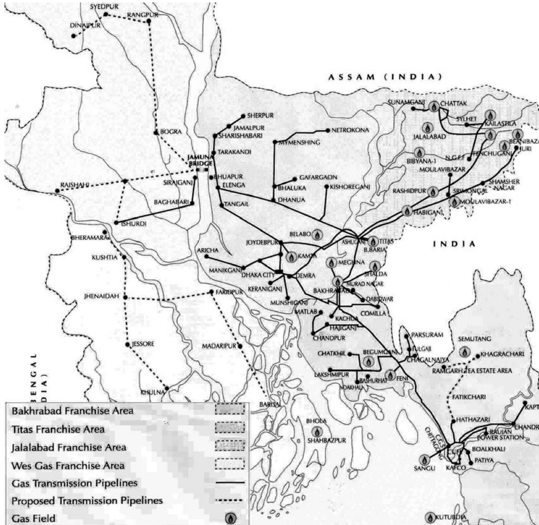
Figure 5.4.4 Gas Pipe Line in Bangladesh
