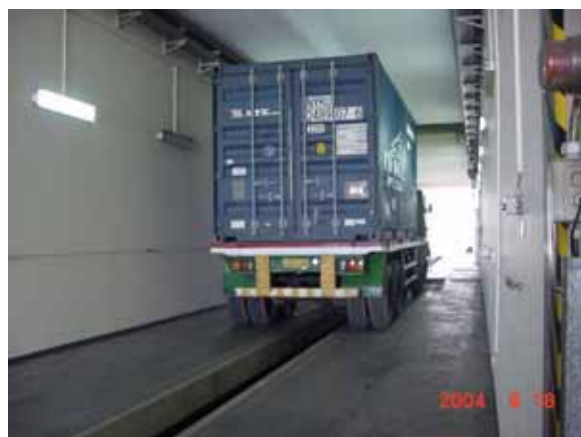
Container Checking Through X ray Booth
