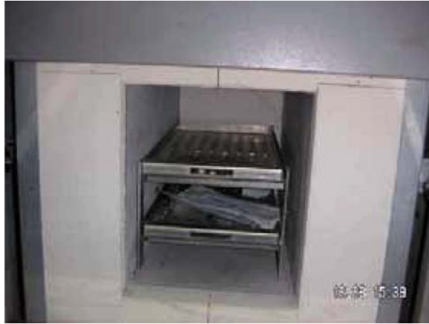
Electric furnace for sterilization of infectious sharps
