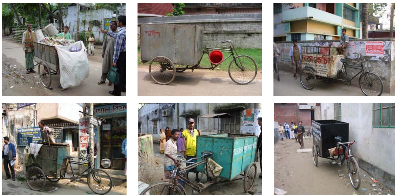
Photo 2.2-1 Various Designs of Rickshaw Vans Used for Primary Collection
