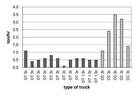
Figure 2.4 Efficiency of Waste Transport by Type of Truck (March 2004, time & motion survey)
