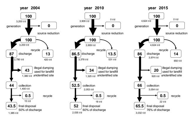
Figure 3.4 Transition of Waste Stream by Target Year (without source reduction)
