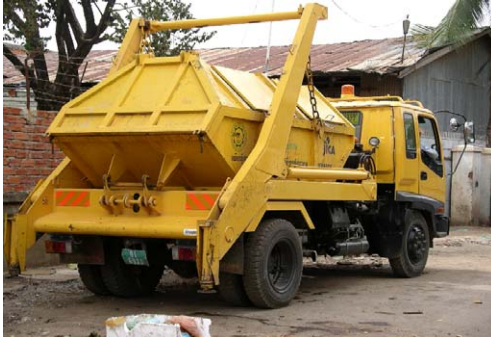
Skip loader truck with 5m 3 container
