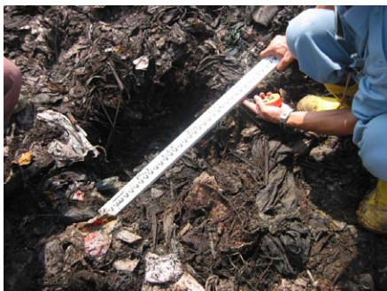
Photo: Measurement of test pit (Width)
