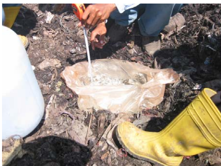
Photo: Measurement of volume of test pit
