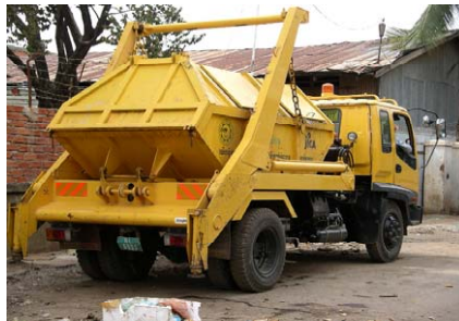
Skip loader truck with 5m 3 container
