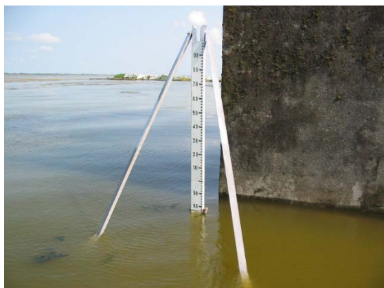
A staff gauge installed in the lagoon to monitor the water level in the wetland.
