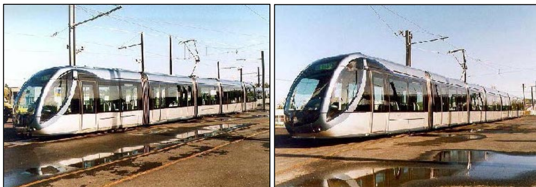
Figure 3.5.24 Example of LRV Extended from 5 to 7 Modules
