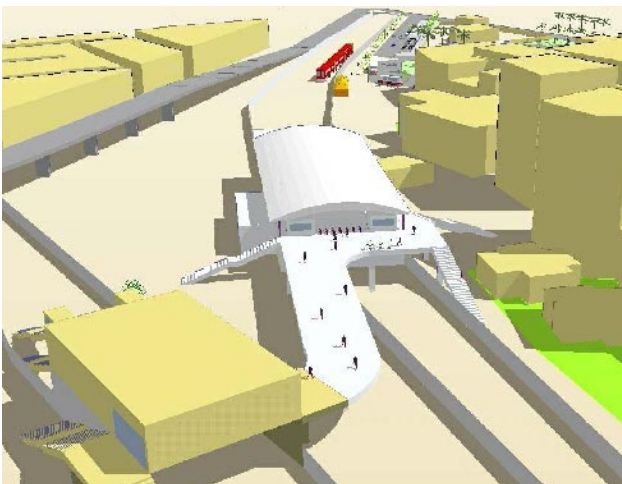
Figure ES.6 Pedestrian Connection between the East Wing Rail and Metro Line1 at Ain Shams
