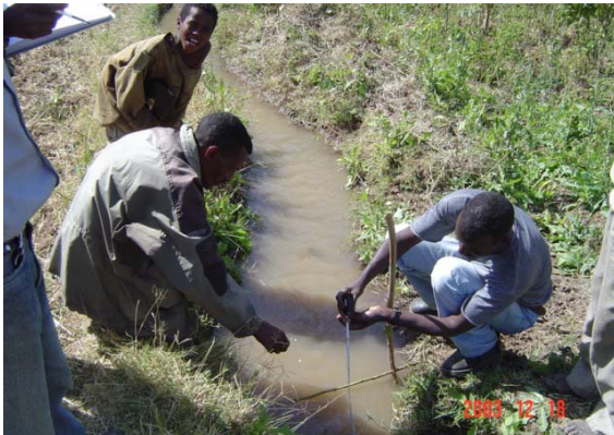
Monitoring of Water Conveyance Loss by OIDA Staff in Shubi-Sombo Schemes (2nd PBME on December 2003)
