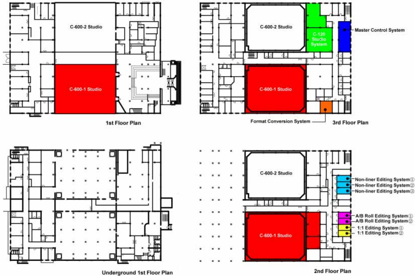
Fig. 2.2-9 NTRC Studio Plan (Underground 1 st Floor, 1 st Floor, 2 nd Floor, 3 rd Floor)
