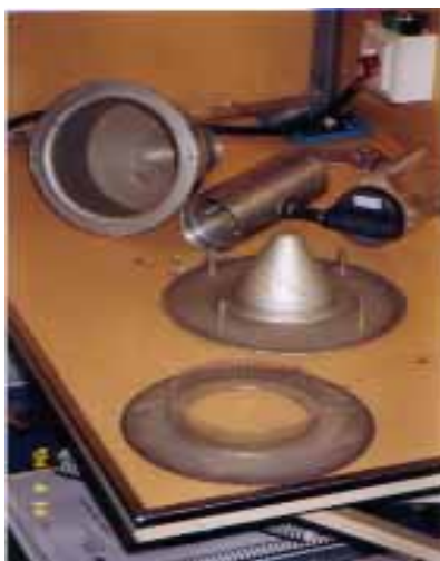
Figure 4.4 Revision and cleaning of a PM 10 head
