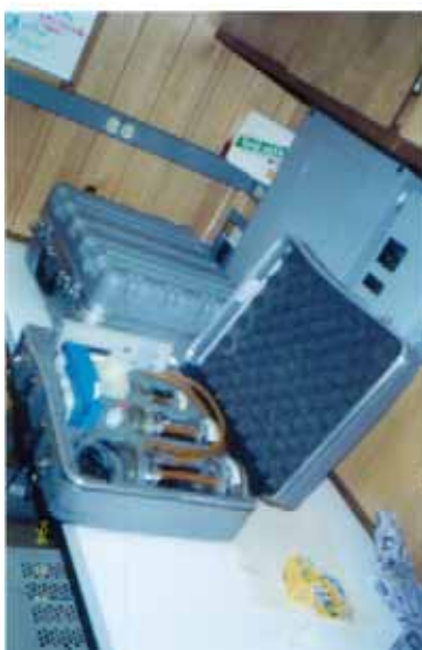
Figure 5.2 Kit for the calibration of flow meters in monitoring stations
