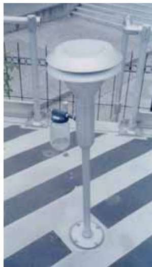
Figure 8 Sample inlet of an automatic particle analyzer
