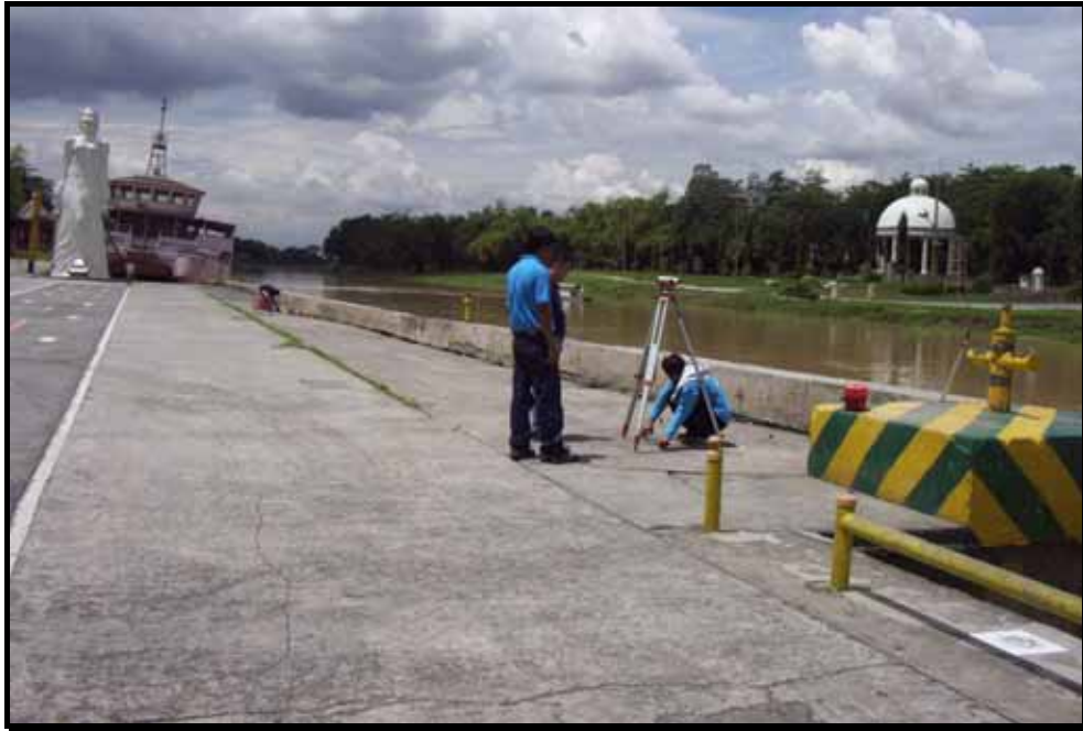
Measuring 30 meter from first observation line up to the second line along the bank of a straight section of the selected river
