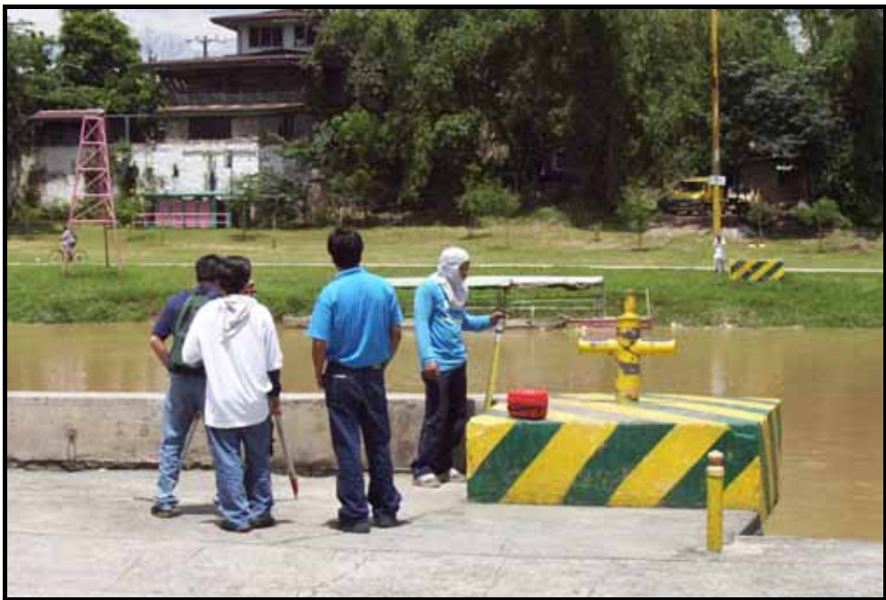
Determining a 90^\circ from the first observation line up to the second observation line and opposite bank
