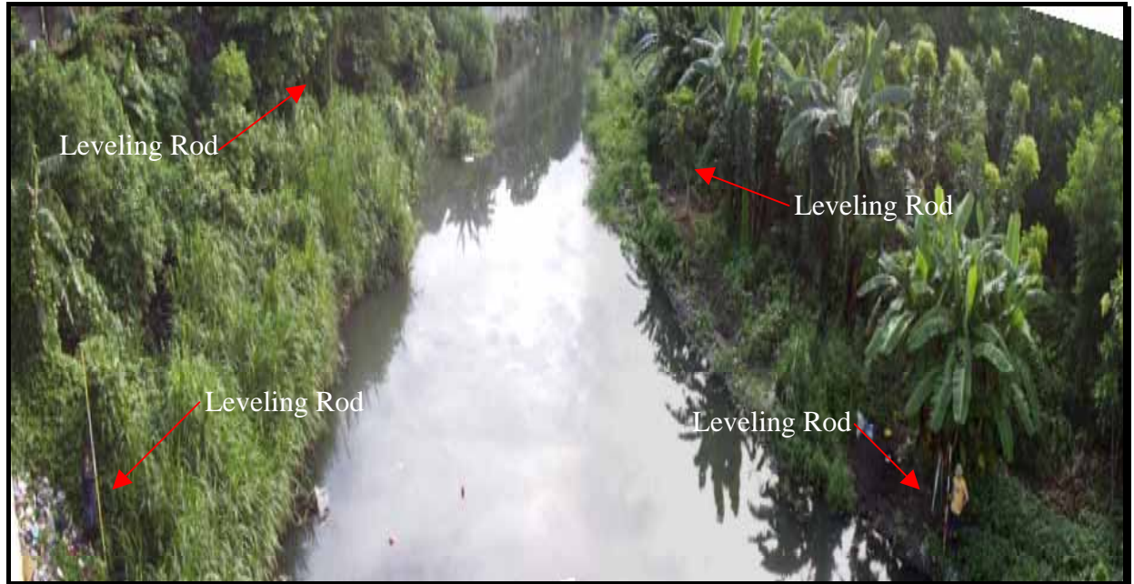
Location of leveling rod, which will serve as starting and end point of the float
