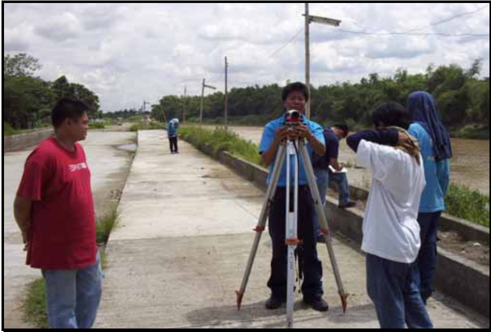
Leveling the bubbles of the transit
