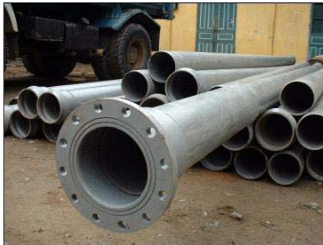
Figure 3-17 PVC pipes (pressure resistant type)
