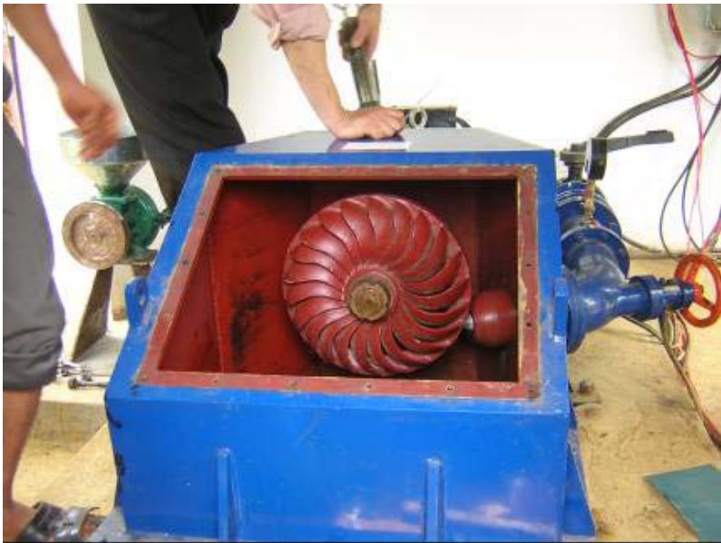
Figure 3-4-1 The Turgo impulse turbine
