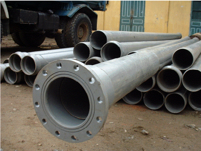
Figure 3-3-10 PVC pipes and a flange joint
