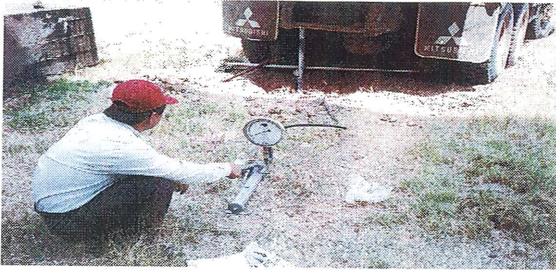
Figure 9. Photographs of Plate Test
