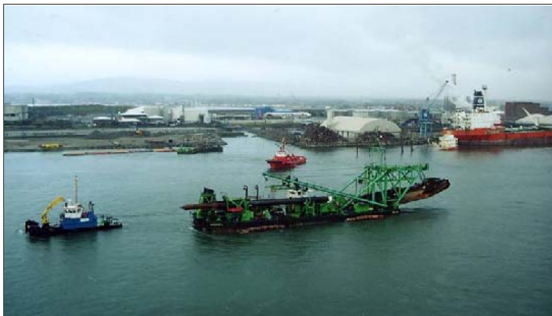
Photo III.6.3-4 Cutter suction dredger
