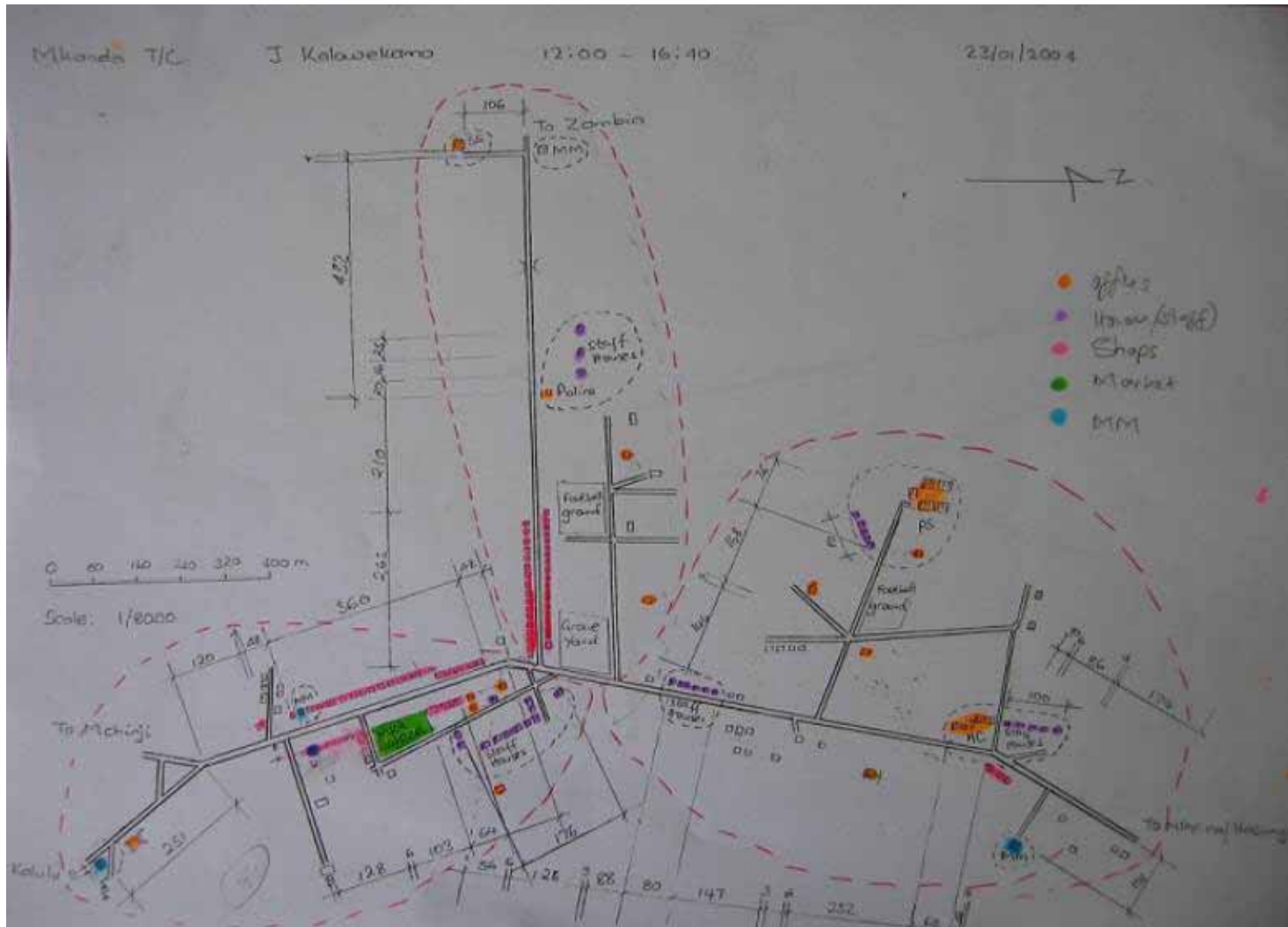
Figure 2-9 Example of Drawing of site situation at Mkanda TC (the procedure determining the supply area of transformer)
