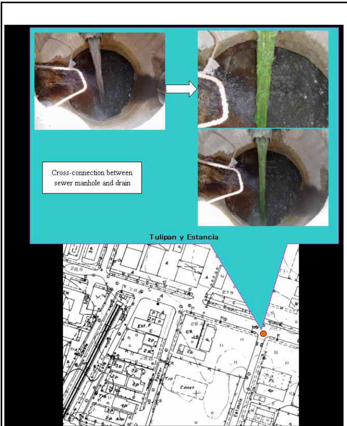
Cross-connection between sewer manhole and drain
