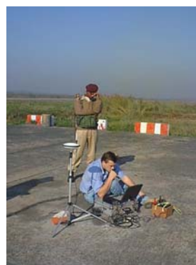
Photo 5.2.4 “GPS Observation for GPS Aerial Photography”
