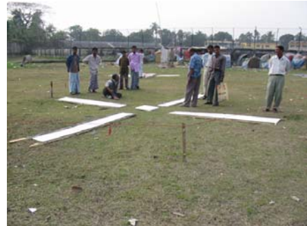
Photo 6.3.1 “Establishment of Photo Signal”
