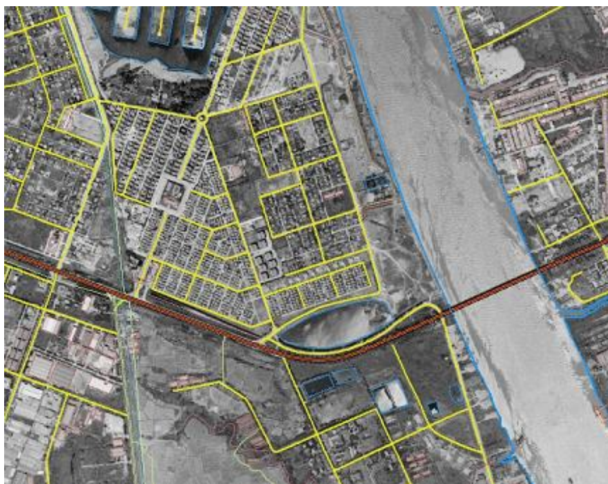
Figure 12.1.1 Topographic map data superimposed on orthophoto
