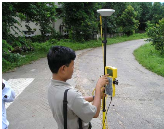
Figure 19.2.2 RTK Survey System (Remote)
