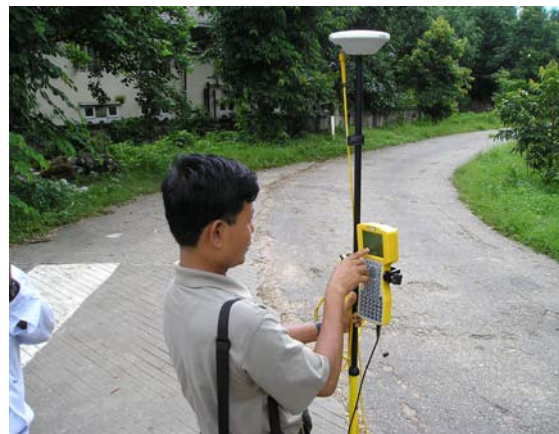
Figure 19.2.2 RTK Survey System (Remote)
