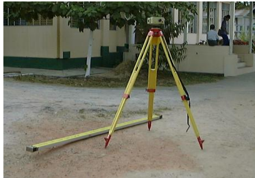
Figure 6.2.3 NA3003 Level and Rod
