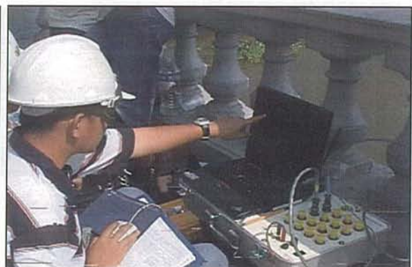
Photo 20.1.3-5 Data acquisition system
