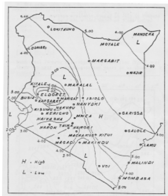
図 3-4 ケニアの風速期待値分布 (出典：Design Manual for Water Supply in Kenya, Ministry of Water Development, 1986)
