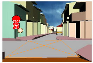
C) Proposed proper traffic signs, safety mirror, yellow box, pedestrian walkway and ramp for handicapped.
