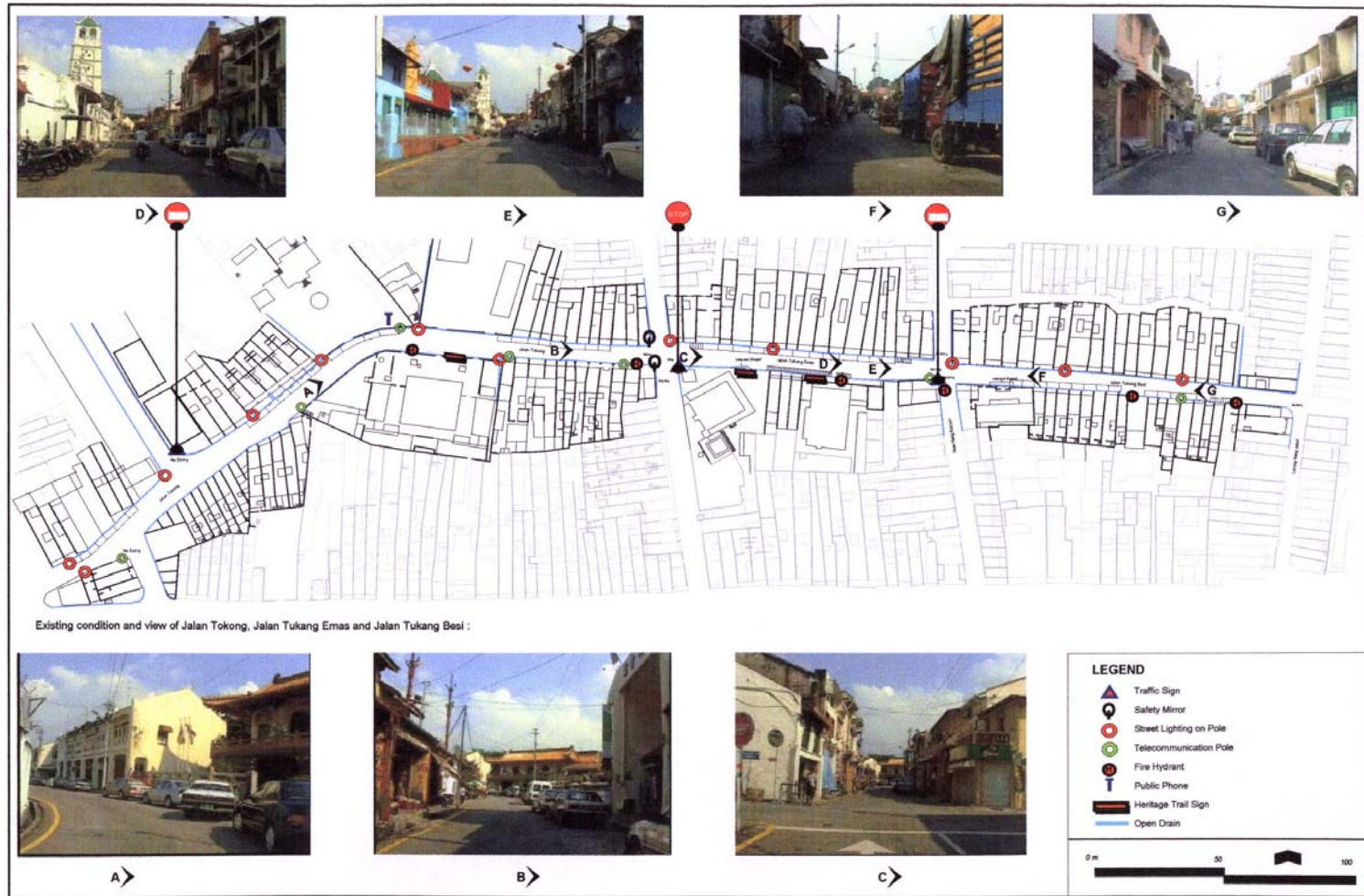
Figure 4.5.3 : Existing Infrastructure Layout Plan
