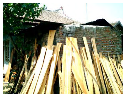
Sun drying of wood (Putting wood against wall makes wood twist)
