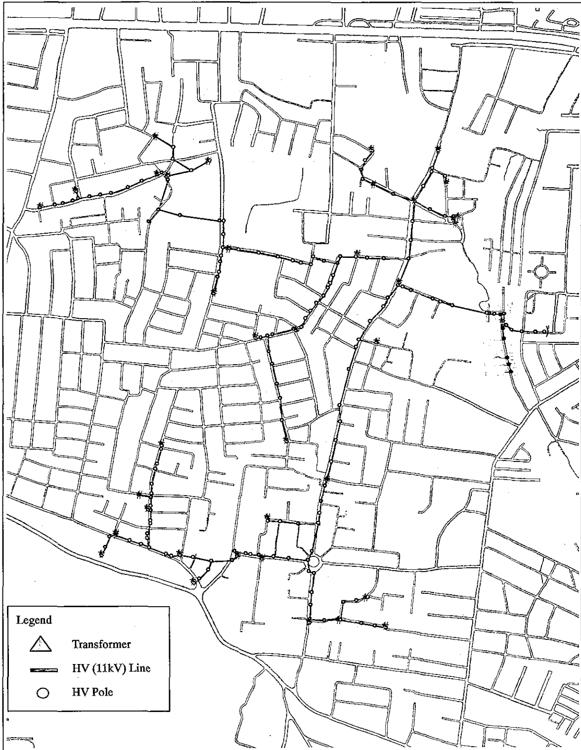
Kothapet substation : Kalamanager feeder
