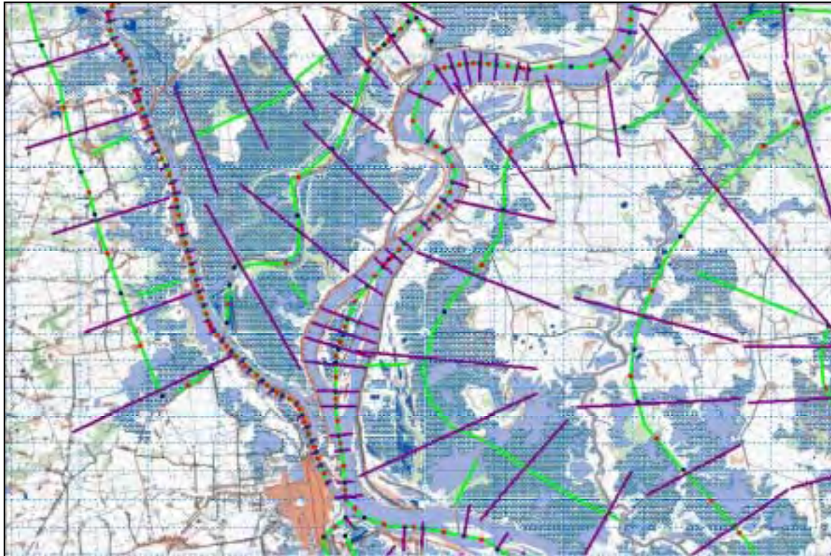
Fig. 3-10 Detailed View of Branch and Cross Section Layout around Phnom Penh Area
