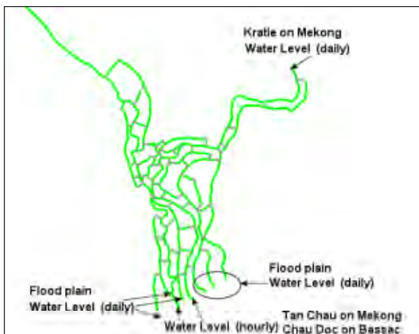
Fig. 3-11 Location and Type of Boundary Conditions Applied
